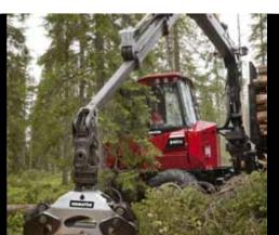
ProTec -Komatsu's unique grapple/ loader tip hose protection system extends hydraulic hose life. ProTec reduces costs and downtime while improving operator productivity.
