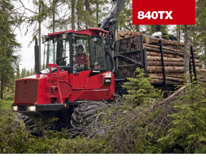
new frame design is 60 cm (2') shorter than its predecessor making it much easier to maneuver. The front axle-to-nose distance, shortened by 25 cm (10") and its 30 cm (12") shorter rear frame-to-articulation joint makes tighter turning a breeze. Minimal stand damage in dense forests, easier driving through ditches and tires that track in the same path make this a very fast and productive forwarder.
